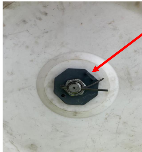
Replacement washer fitted to sheave
